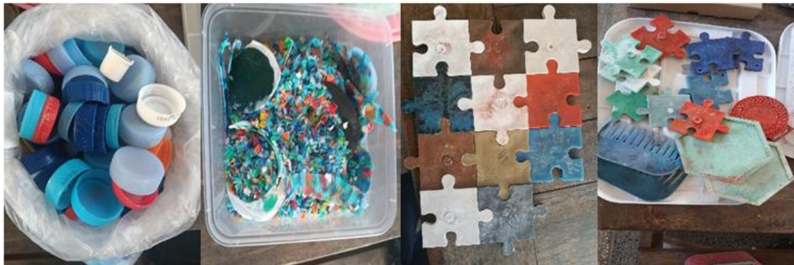
Figure 3. Processing of plastic waste into shredded plastic and recycled product
